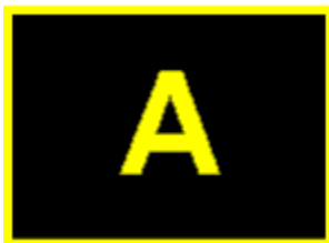
Taxiway Location Sign
