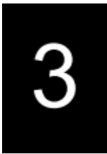
Runway Distance Remaining Signs
