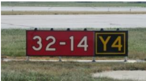
Runway Hold Sign
