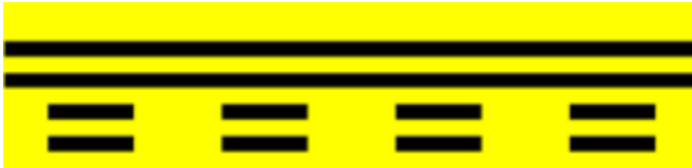
Runway Safety Area/OFZ and Runway Approach Boundary Sign
